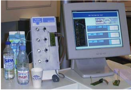
Fig. 9 The water test demonstrator. The different mineral waters enter the pinch valve board on the left, the liquid flows through the cell (attached on the valve board). The sensor signals are entered in the computer and processed on the screen (ACHEMA2000).
