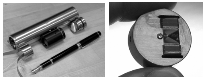
Figure 3: Free-space WDM optomechanics, showing header, 50mm focal length lens and 600 lp/mm grating. At right, a close-up of the device, electrical flex-circuit contacts, and I/O fiber ferrule on the cylindrical metal header.
